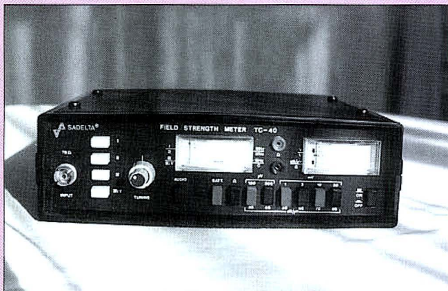
Fig. 1: Designed originally for domestic v.h.f. radio and TV signal strength metering, this f.s.m. from Sadelta is nonetheless very useful for amateur frequencies.
