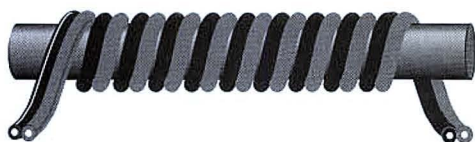
Fig. 2: A ferrite rod filter (see text).
