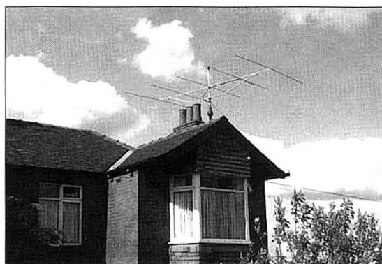
Fig. 2: The 50MHz antenna used by G0DJJA.
